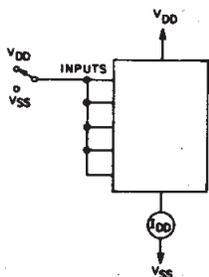
Fig. 11 - Quiescent device current test circuit.
