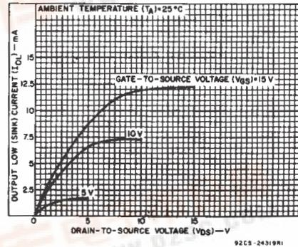
Fig.2 - Minimum output low (sink) current characteristics.
