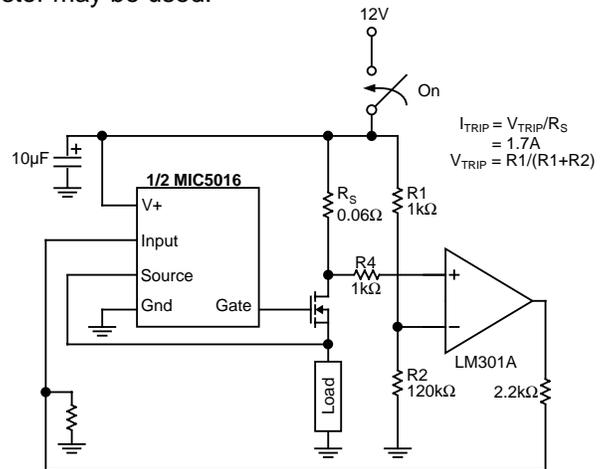
Figure 4. High Side Driver with Overcurrent Shutdown
