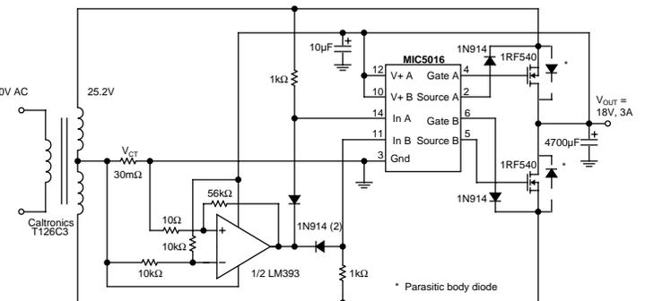
Figure 14: High Efficiency 60 Hz Synchronous Rectifier
