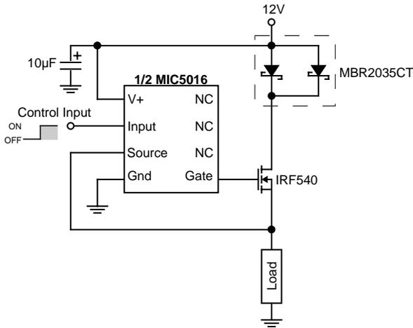
Figure 12: High Side Driver With Load Protection
