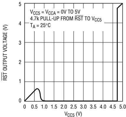
**Figure 4.  $\overline{\text{RST}}$  Output Voltage Characteristics of the Circuit in Figure 3**
