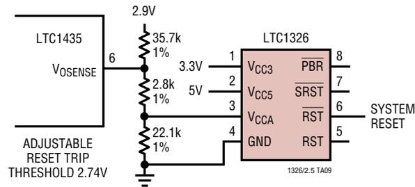
**Using the Short Pulse Width, Push-Button Soft Reset Feature to Initiate Hard Reset**
