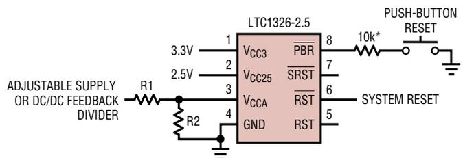
\*OPTIONAL RESISTOR EXTENDS ESD TOLERANCE OF  $\overline{\text{PBR}}$  INPUT TO APPROXIMATELY 10KV 1326/2.5 F05
