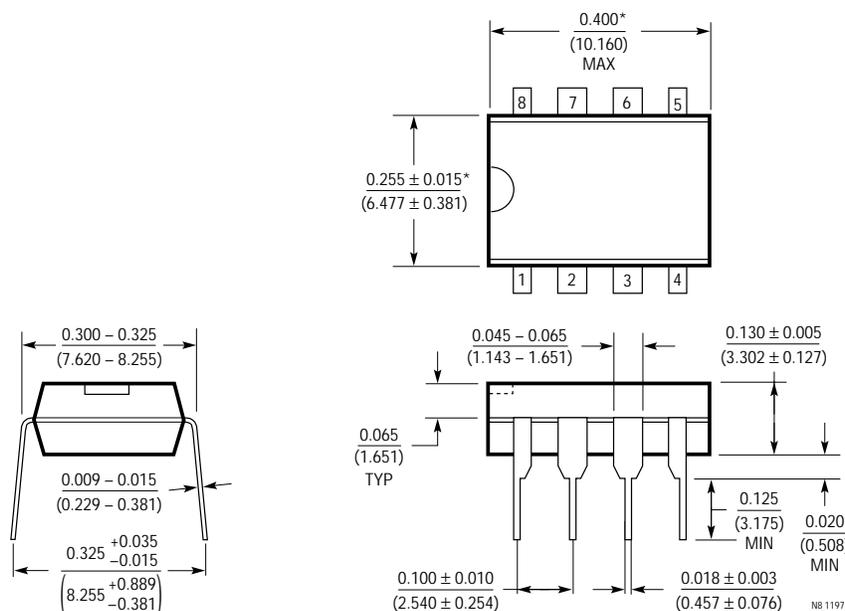
\*THESE DIMENSIONS DO NOT INCLUDE MOLD FLASH OR PROTRUSIONS.
