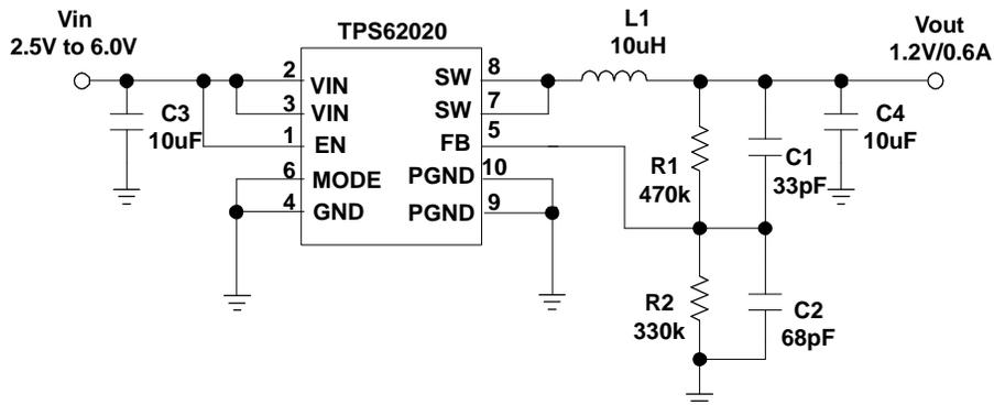
Figure 19. 1.2 V Output Using 10  $\mu$ H Inductor
