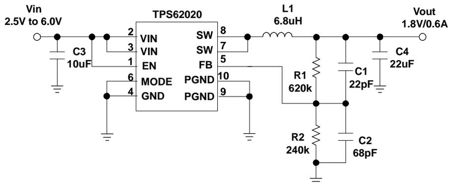
Figure 18. 1.8 V Output Using 6.8  $\mu$ H Inductor
