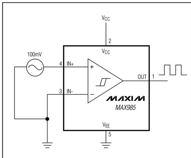
Figure 3. Zero-Crossing Detector
