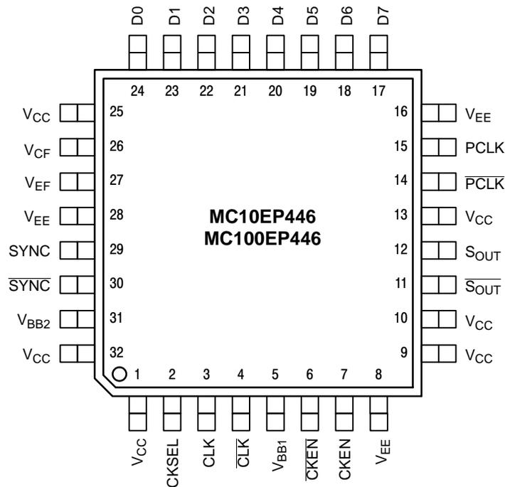
Warning: All  $V_{CC}$  and  $V_{EE}$  pins must be externally connected to Power Supply to guarantee proper operation.
