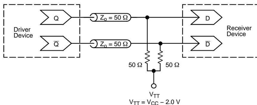
**Figure 16. Typical Termination for Output Driver and Device Evaluation**
