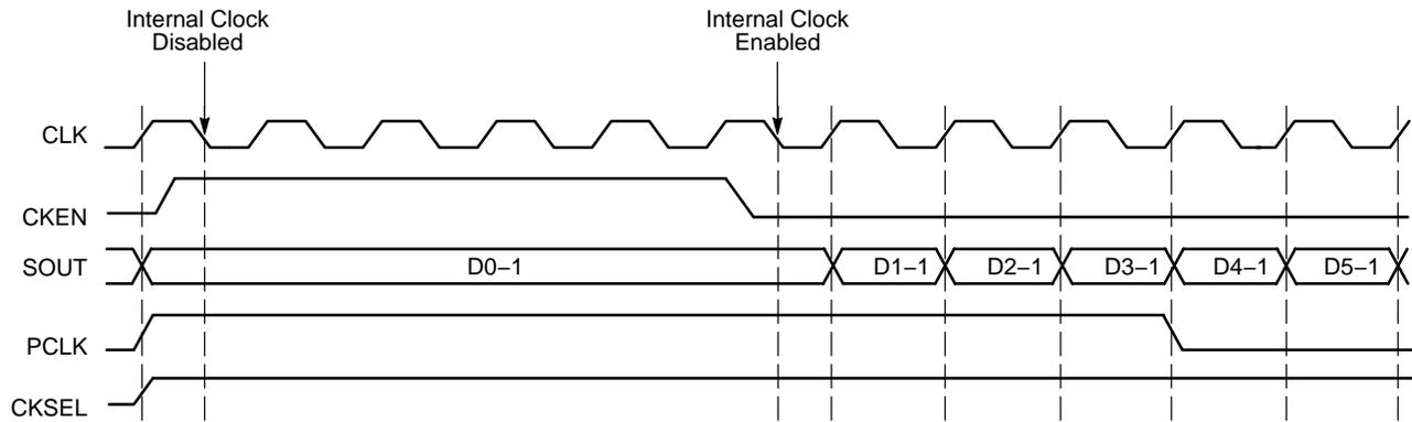
Figure 12. Timing Diagram with CKEN with CKSEL HIGH
