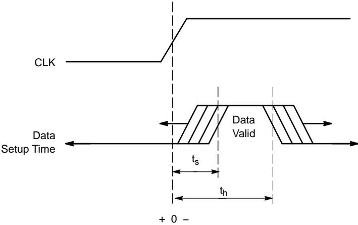
**Figure 3. Setup and Hold Time for Data**
