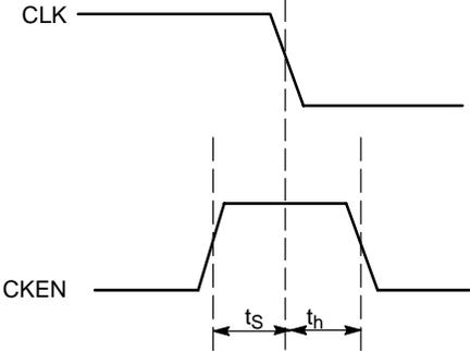
**Figure 5. Setup and Hold Time for CKEN**
