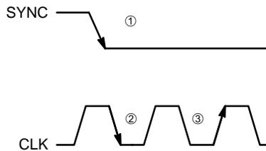
Figure 11. Synchronous Release of SYNC for CKSEL HIGH
