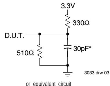
**Figure 1. Output Load**
