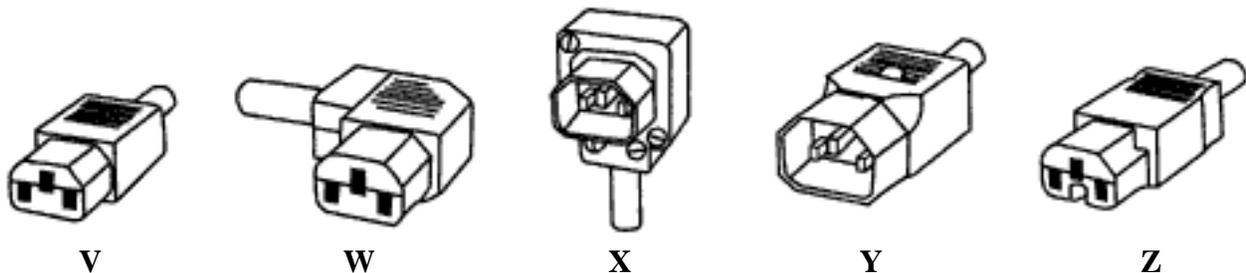
Male and Female rewirable plug connectors with straight and 90° angle cable entry. Easily converts a power cord into a detachable power cordset.
