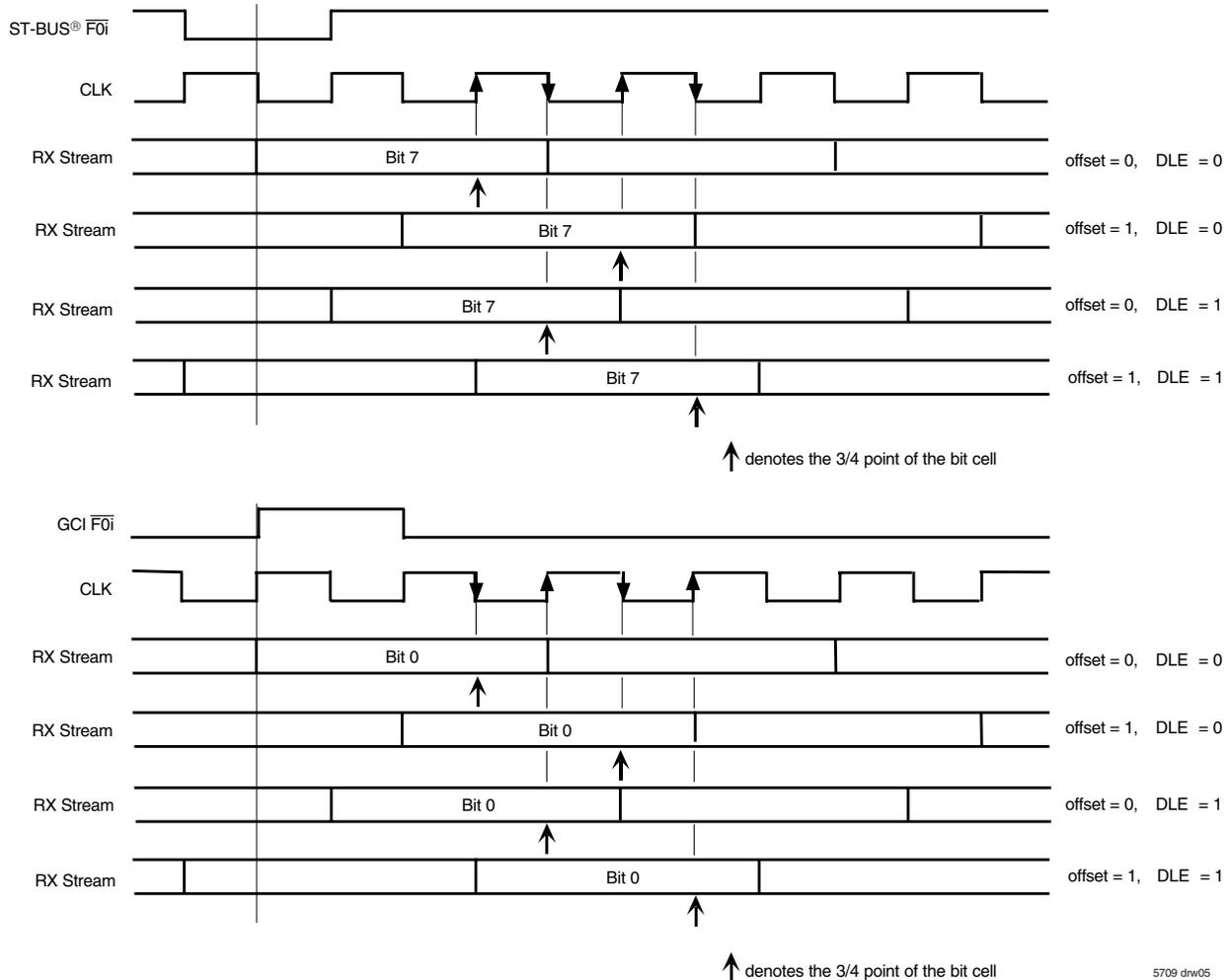
Figure 5. Examples for Input Offset Delay Timing
