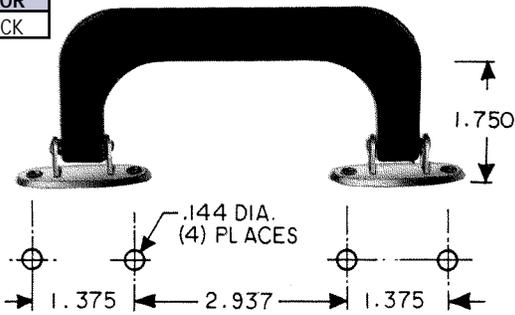
Molded of high impact styrene with steel nickel plated hardware. Folds flat on case when not in use. Mounts with #10-32 screws (not supplied)
