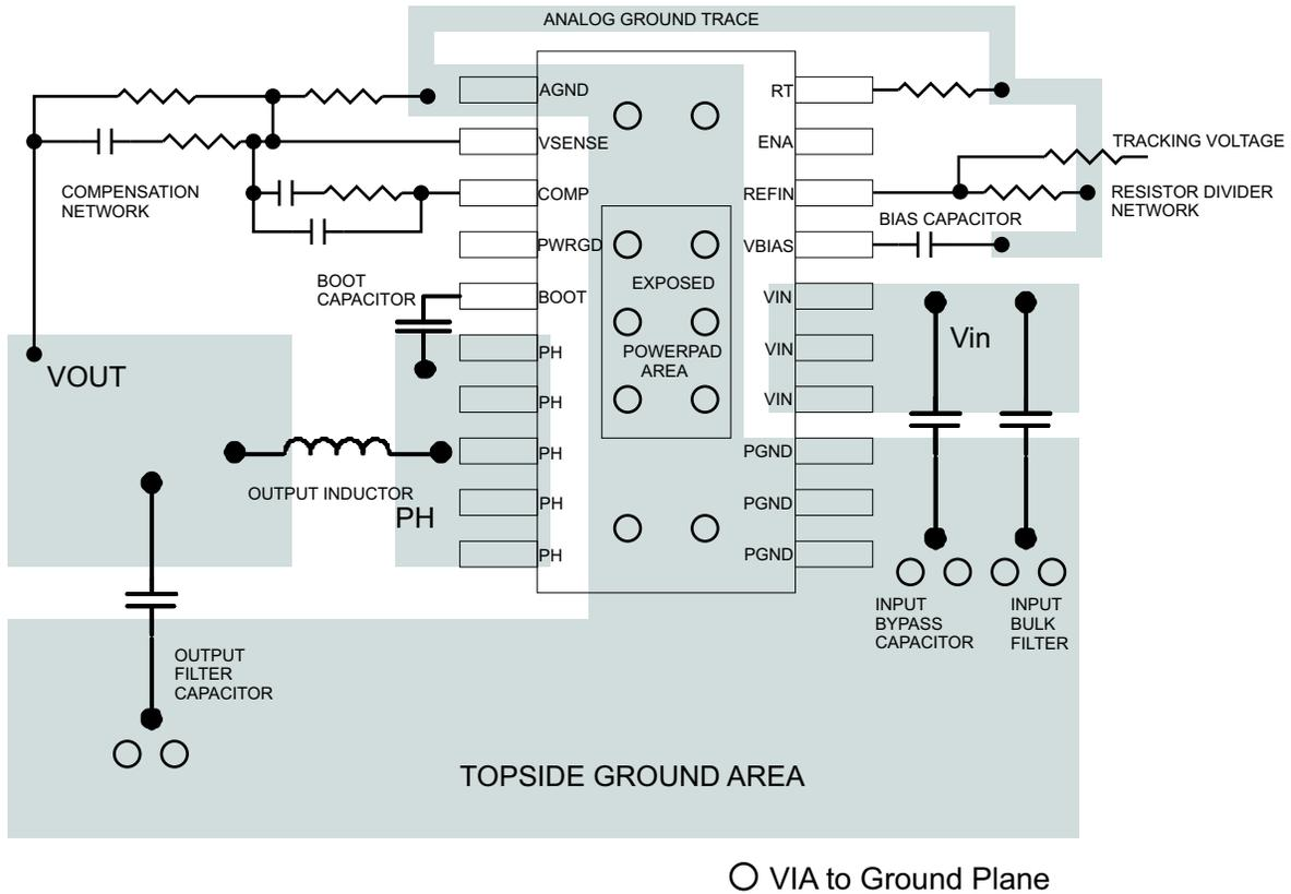
Figure 9. PCB Layout for 20-Pin PWP PowerPAD
