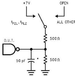
\*Includes jig and probe capacitance.
