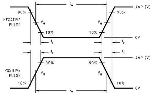
**FIGURE 2.  $V_M = 1.5\text{V}$**
