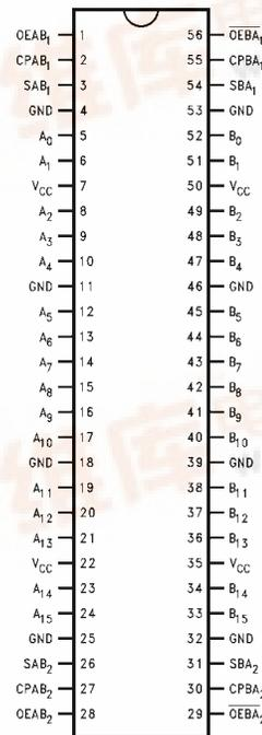
74ABT16652 16-Bit Transceivers and Registers with 3-STATE Outputs
