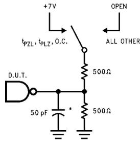
\*Includes jig and probe capacitance
