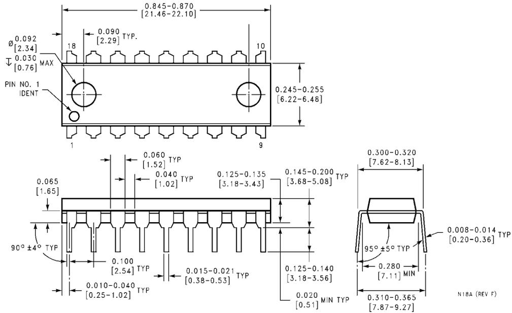
**18-Lead Plastic Dual-In-Line Package (PDIP), JEDEC MS-001, 0.300" Wide
