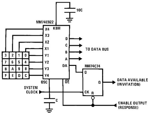
The keyboard may be synchronously scanned by omitting the capacitor at osc. and driving osc. directly if the system clock rate is lower than 10 kHz
