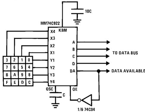
Outputs are in 3-STATE until key is pressed, then data is placed on bus. When key is released, outputs return to 3-STATE.
