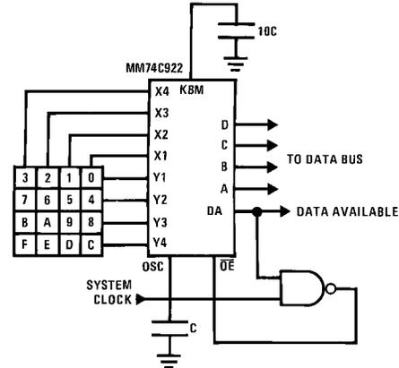
Outputs are enabled when valid entry is made and go into 3-STATE when key is released.
