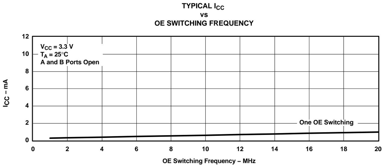
Figure 2. Typical  $I_{CC}$  vs OE Switching Frequency
