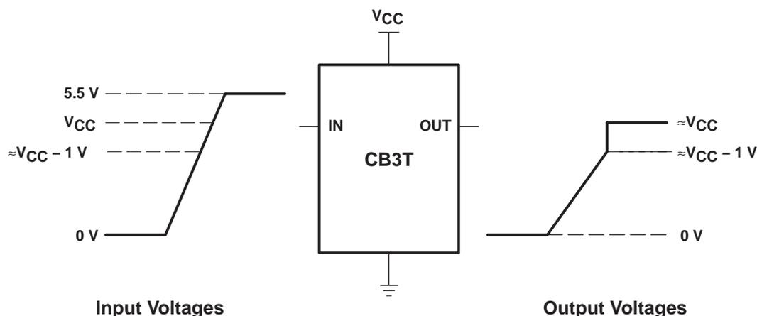
NOTE A: If the input high voltage ( $V_{IH}$ ) level is greater than or equal to  $V_{CC} - 1\text{ V}$ , and less than or equal to 5.5 V, the output high voltage ( $V_{OH}$ ) level will be equal to approximately the  $V_{CC}$  voltage level.
