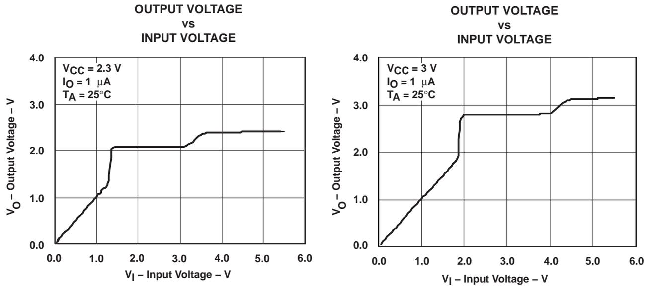
Figure 3. Data Output Voltage vs Data Input Voltage
