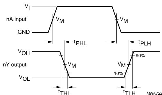
For 74HC04:  $V_M = 50\%$ ;  $V_I = \text{GND to } V_{CC}$ .For 74HCT04:  $V_M = 1.3 \text{ V}$ ;  $V_I = \text{GND to } 3.0 \text{ V}$ .
