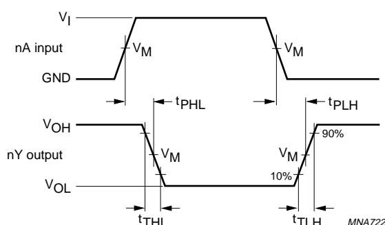
74HC14:  $V_M = 50\%$ ;  $V_I = \text{GND to } V_{CC}$ .74HCT14:  $V_M = 1.3$  V;  $V_I = \text{GND to } 3.0$  V.
