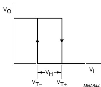
Fig.7 Transfer characteristic.
