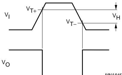
$V_{T+}$  and  $V_{T-}$  are between limits of 20% and 70%.Fig.8 The definitions of  $V_{T+}$ ,  $V_{T-}$  and  $V_H$ .
