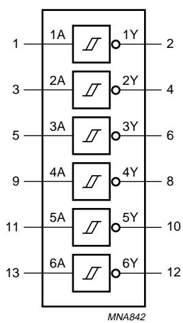
Fig.5 Functional diagram.
