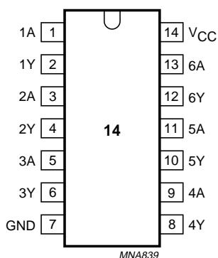
Fig.1 Pin configuration.
