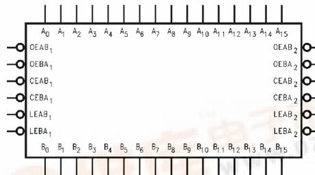
74LCX16543 Low Voltage 16-Bit Registered Transceiver with 5V Tolerant Inputs and Outputs
