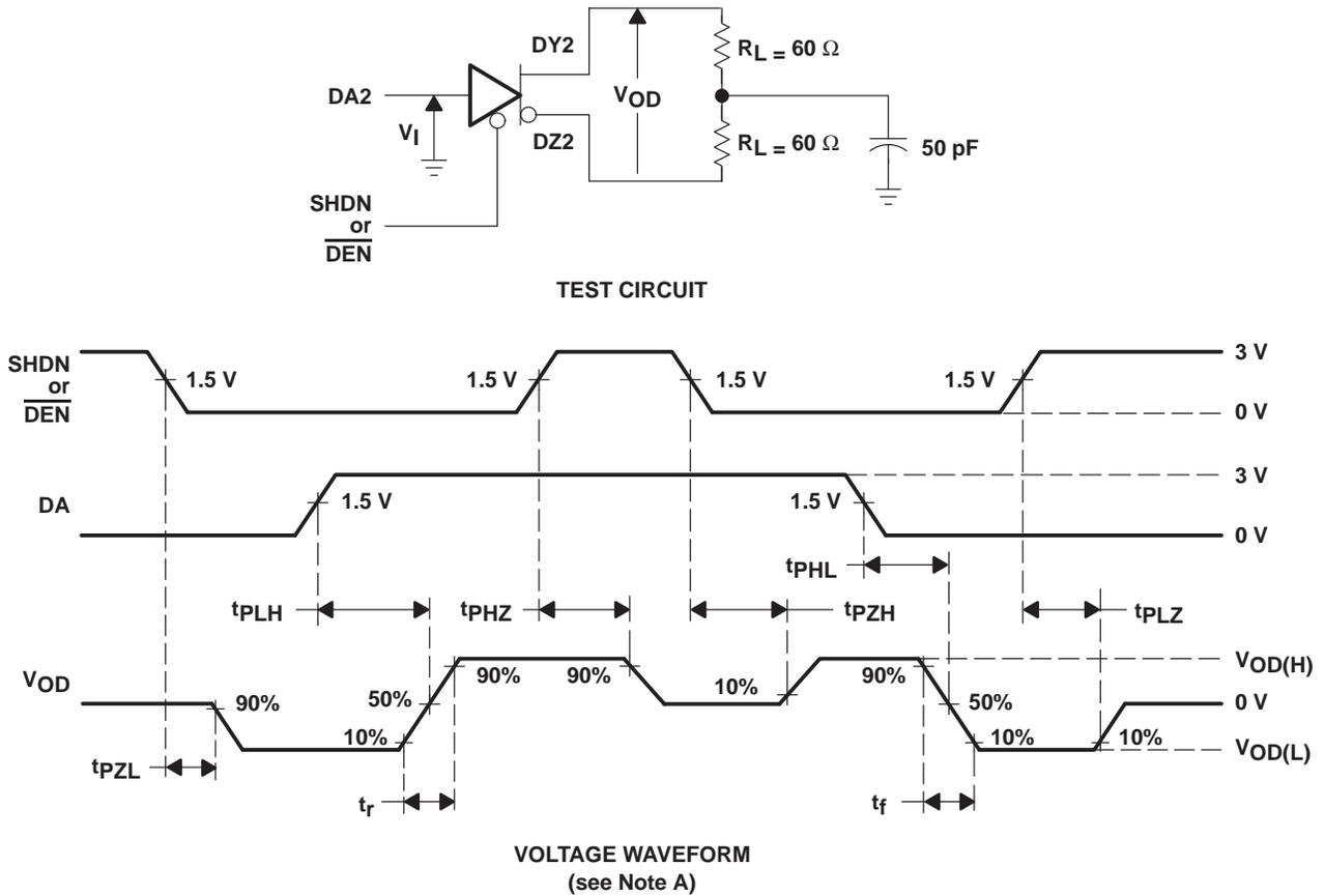
Figure 5. Differential Driver Propagation and Transition Times
