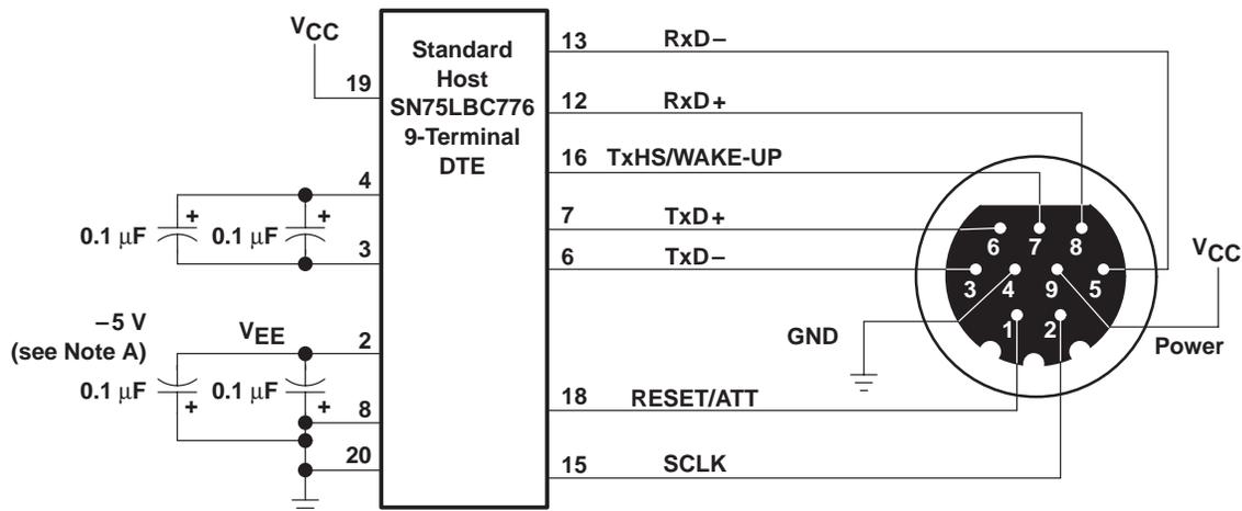
NOTE A: The AVX 0603YC104MATXA or equivalent is one of the possible capacitors that can be used as the charge pump capacitor.
