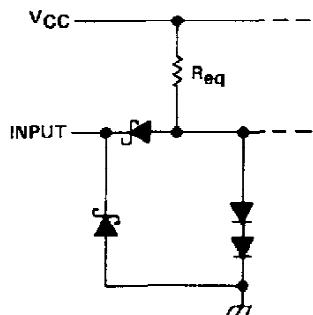
Data select and strobe  $R_{eq} = 20 \text{ k}\Omega \text{ NOM}$
