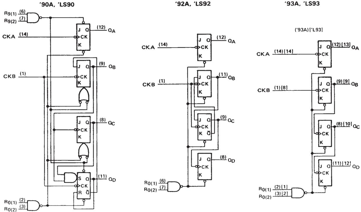
The J and K inputs shown without connection are for reference only and are functionally at a high level.
