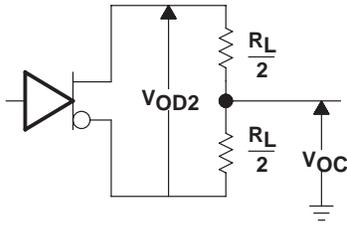
Figure 1. Driver Test Circuit,  $V_{OD}$  and  $V_{OC}$
