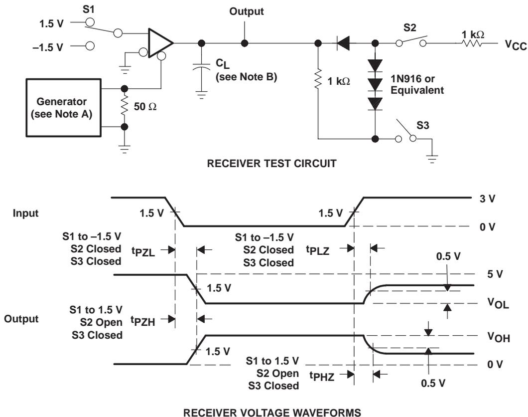
NOTES: A. The pulse generator has the following characteristics:  $PRR \leq 1$  MHz, 50% duty cycle,  $t_r \leq 10$  ns,  $t_f \leq 10$  ns.
