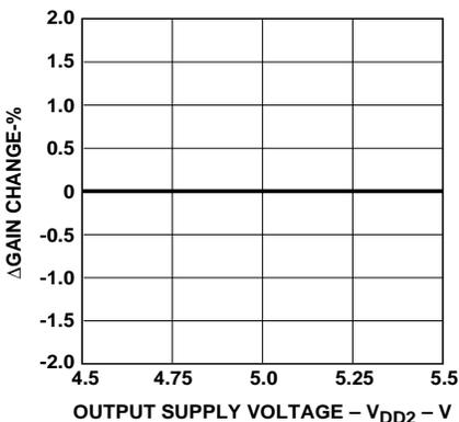
Figure 9. Gain Change vs.  $V_{DD2}$ .
