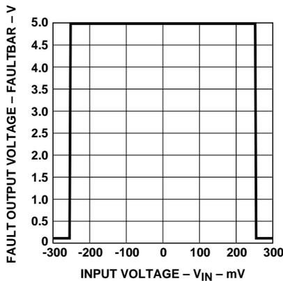
Figure 10. FAULT Output Voltage vs.  $V_{IN}$ .
