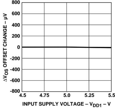
Figure 4. Input Offset Voltage Change vs.  $V_{DD1}$ .
