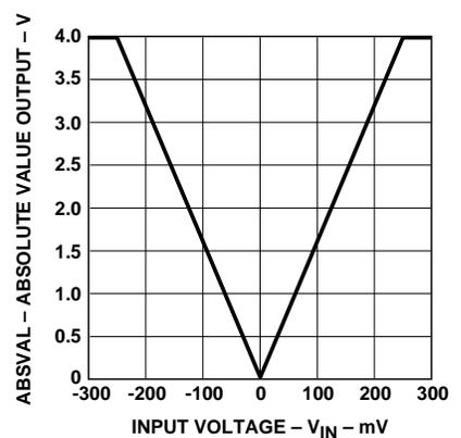
Figure 11. ABSVAL Output Voltage vs.  $V_{IN}$ .
