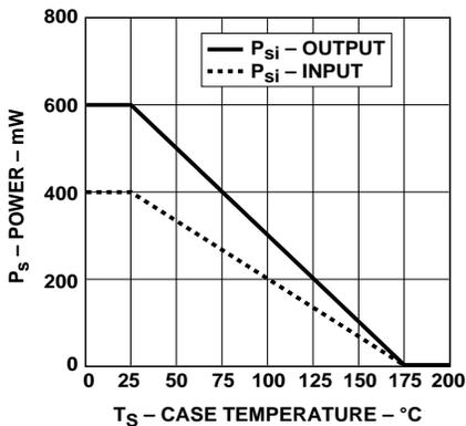
Figure 2. Dependence of Safety-Limiting Values on Temperature.
