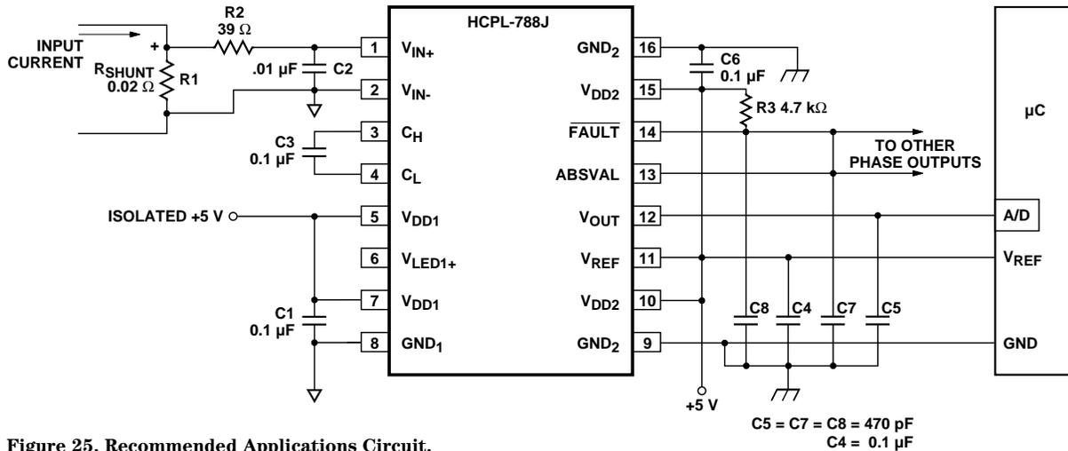
Figure 25. Recommended Applications Circuit.
