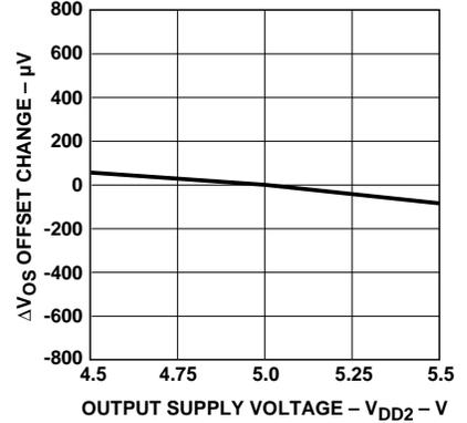
Figure 5. Input Offset Voltage Change vs.  $V_{DD2}$ .
