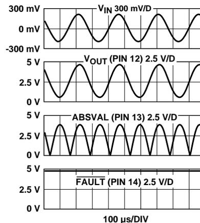
Figure 19. Sine Response 400 mV pk to 300 mV Input, at  $V_{REF} = 5$  V.
