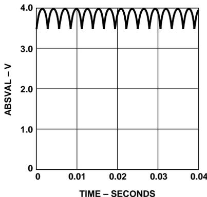
Figure 22. ABSVAL with 3 Phases, Wired-ORed Together.
