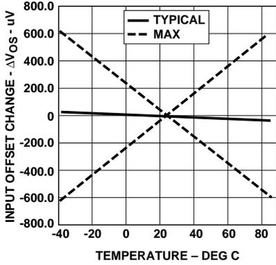
Figure 3. Input Offset Voltage Change vs. Temperature.
