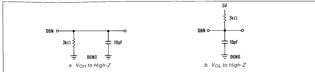
Figure 2. Load Circuits for Bus Relinquish Time
