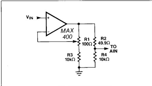
Figure 16. Trim Circuit for Gain Only ( $\pm 0.5\%$ )
