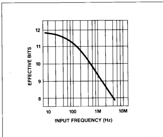
Figure 19. MAX167 Effective Bits vs. Input Frequency
