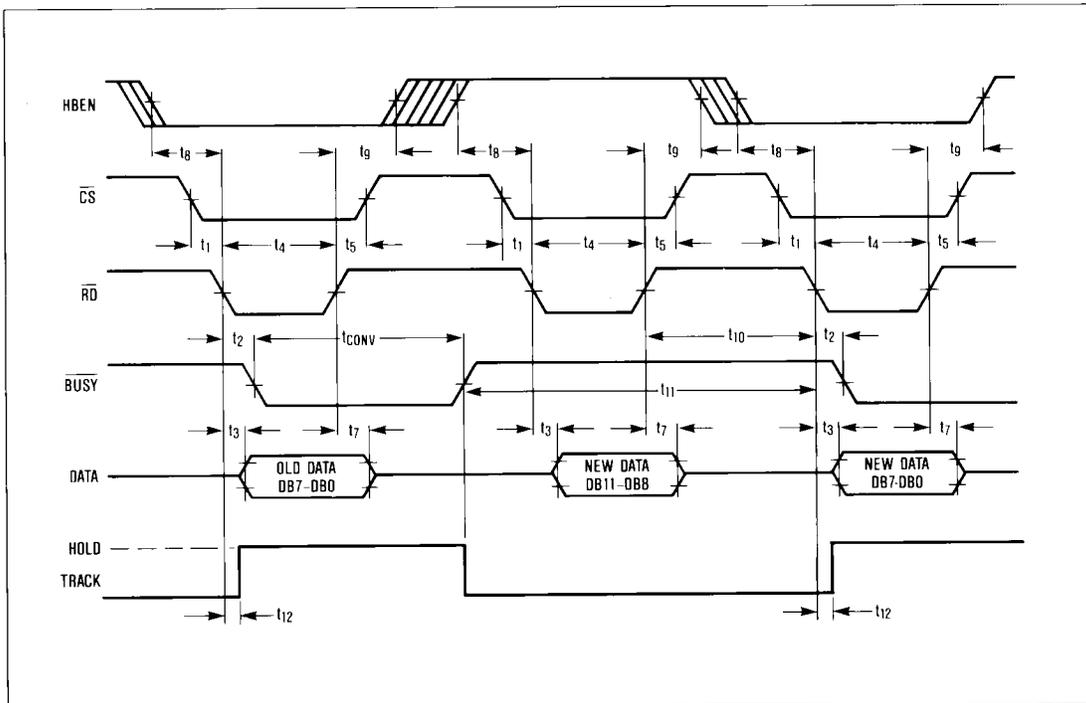
Figure 12. ROM Mode, Two Byte Read Timing Diagram
