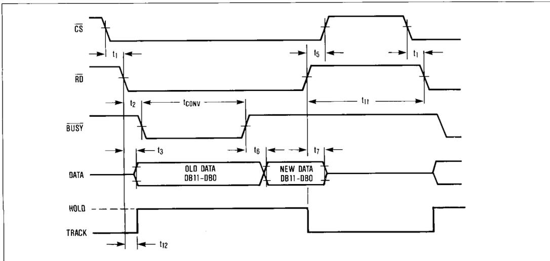
Figure 9. Slow Memory Mode, Parallel Read Timing Diagram
