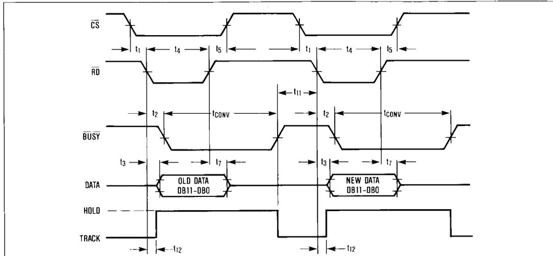
Figure 11. ROM Mode, Parallel Read Timing Diagram
