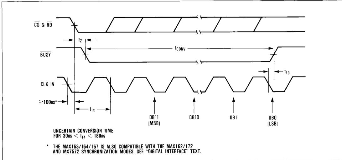
Figure 7.  $\overline{\text{RD}}$  and CLK IN for Synchronous Operation
