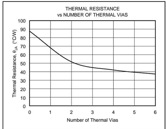
FIGURE 11. Thermal Resistance vs Number of Thermal Vias.
