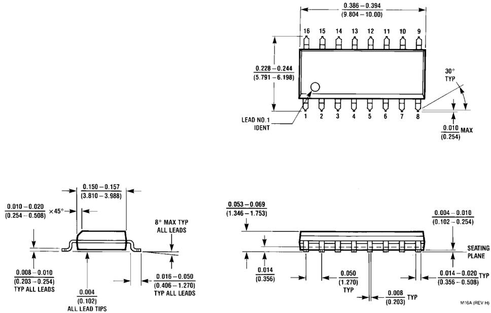
**16-Lead Small Outline Integrated Circuit (SOIC), JEDEC MS-012, 0.150" Narrow Body
