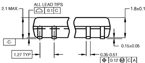
DIMENSIONS ARE IN MILLIMETERS
