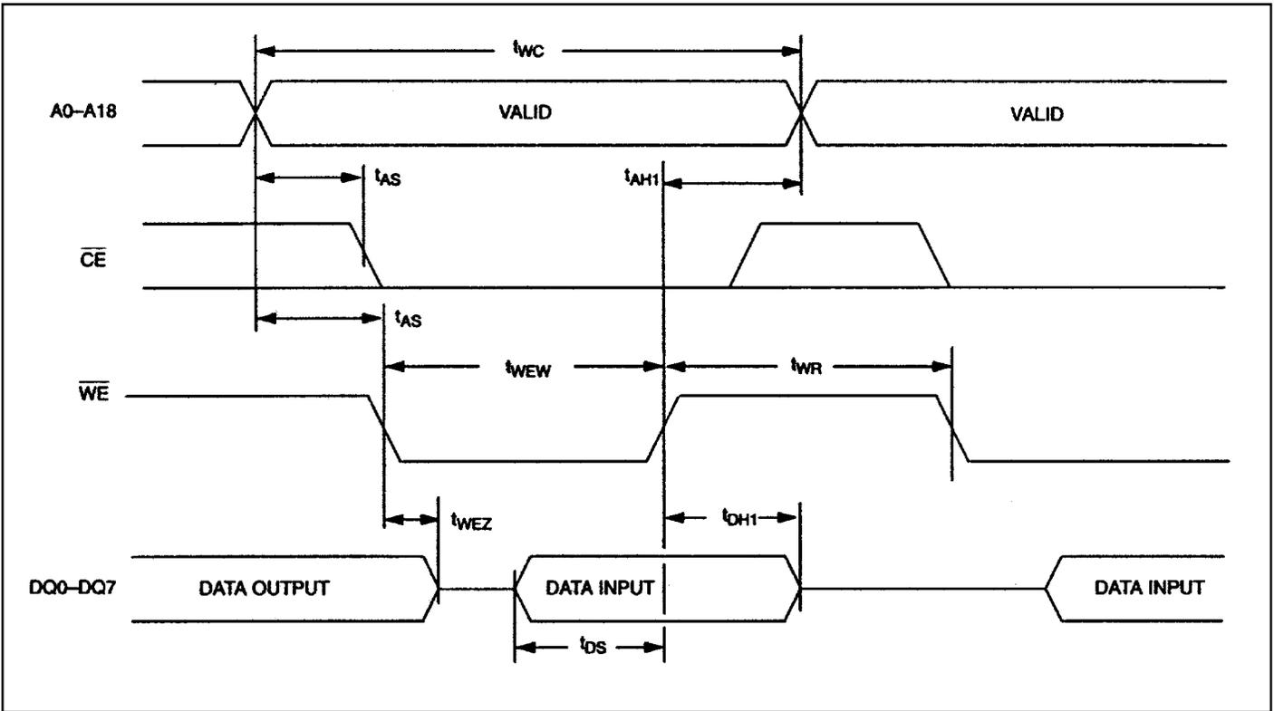
**WRITE CYCLE TIMING DIAGRAM, CHIP-ENABLE CONTROLLED**
