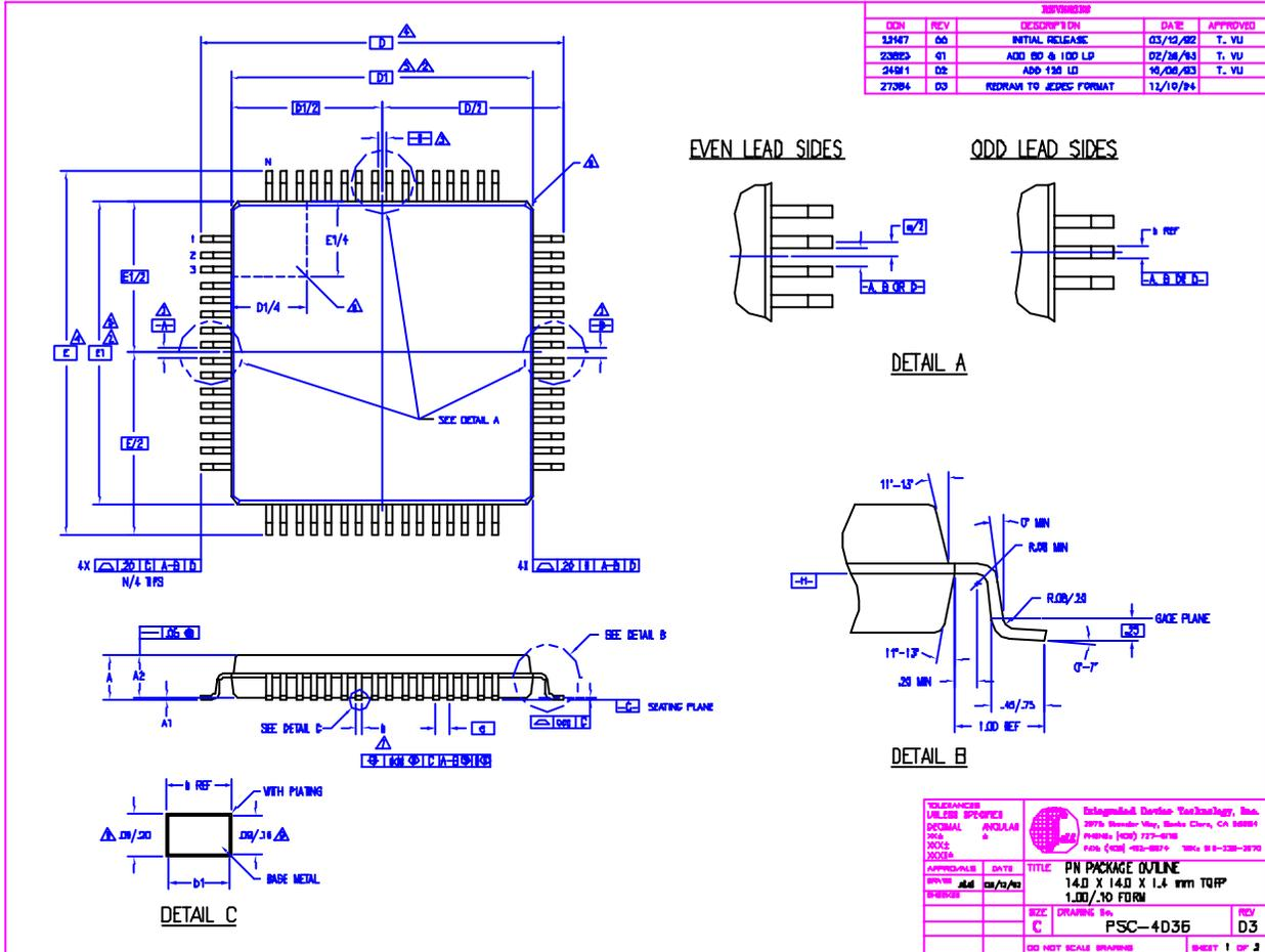
77V500 Package Drawing — 100-pin TQFP (Page Two)
