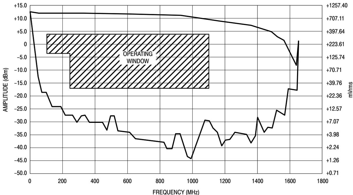
Figure 3. Input Signal Amplitude versus Input Frequency
