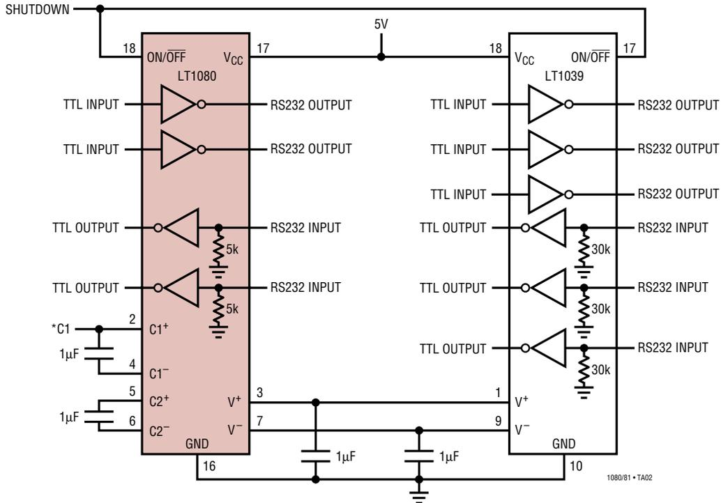
\*IN APPLICATIONS WHERE A SEPARATE SECOND POSITIVE SUPPLY IS AVAILABLE (SUCH AS 5V AND 12V), THE 12V SUPPLY MAY BE CONNECTED TO PIN 2 AND C1 DELETED. THE POWER SUPPLY CIRCUITRY WILL THEN INVERT THE 12V SUPPLY. THE 5V SUPPLY IS STILL NEEDED TO POWER THE BIASING CIRCUITRY AND RECEIVERS.
