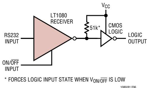
To protect against receiver input overloads in excess of  $\pm 30V$ , a voltage clamp can be placed on the data line and still maintain RS232 compatibility.
