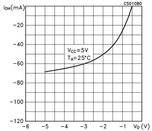
**Figure 10 : Receiver Output Current vs Output High Voltage**
