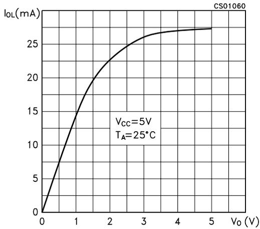
**Figure 12 : Driver Output Current vs Output High Voltage**
