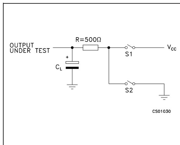
Figure 5 : Driver Propagation Delay
