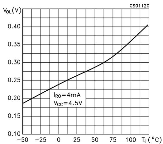
**Figure 16** : Differential Driver Output Voltage vs Temperature
