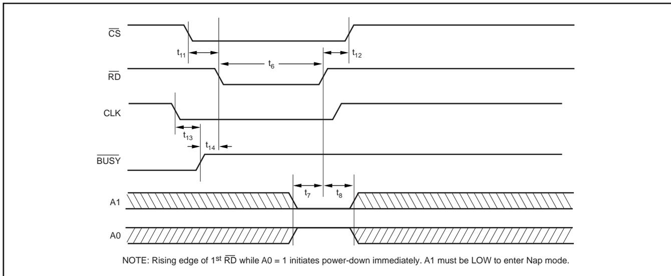
FIGURE 3. Entering Nap Using  $\overline{RD}$  and A0.
