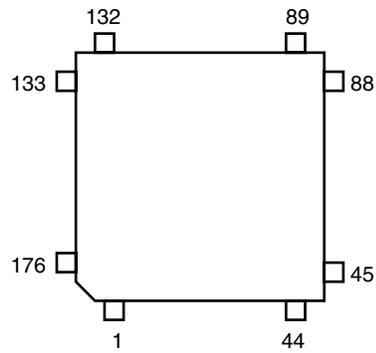
**Figure 2.** 176-ball BGA Pinout
