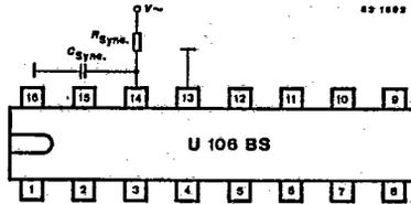
Fig. 8 Pulse delay circuit
