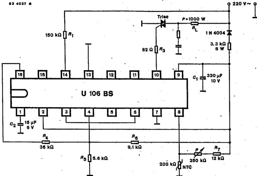
Fig. 24 Temperature control with superimposed proportional characteristic for a temperature range 30...110 °C and  $\pm 3$  °C hysteresis.
