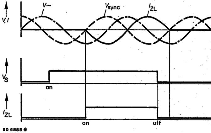
Fig. 22 Optimum switching of inductive loads
