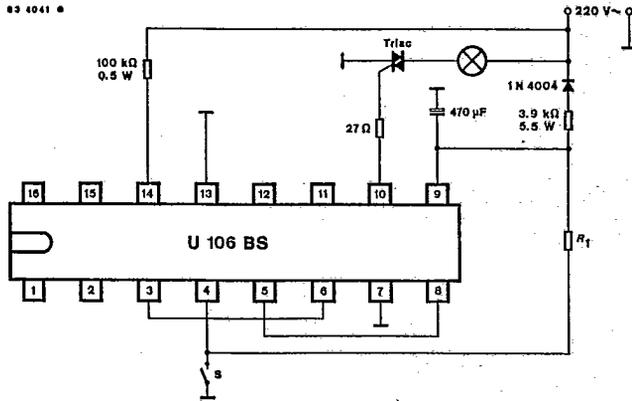
Fig. 28 Static switch
