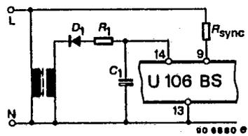
Fig. 5 Mains transformer (low voltage) supply voltage regulator
