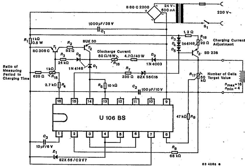
Fig. 29 Automatic charging unit for NC accumulators
