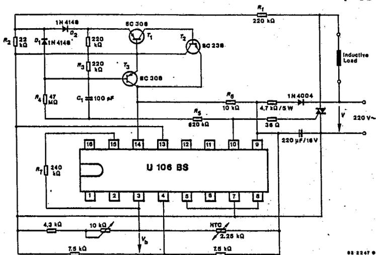
Fig. 23 Two-point temperature control circuit for inductive load
