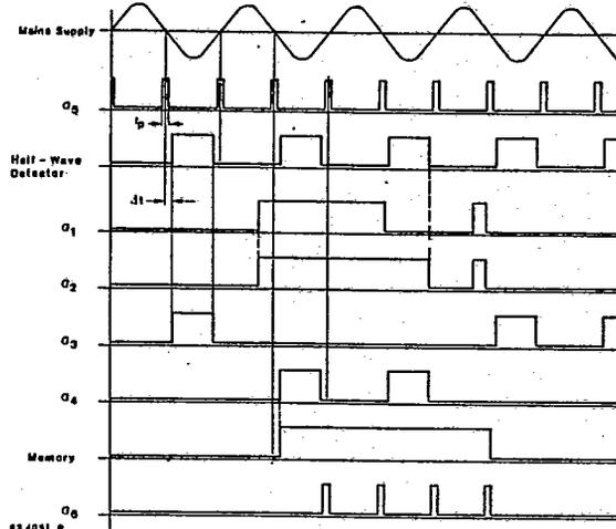
Fig. 10 Pulse diagram of the full-wave logic
