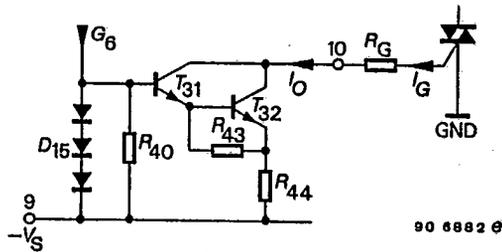
Fig. 11: Firing pulse output
