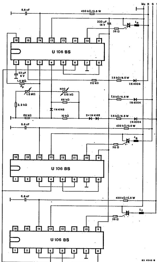
Fig. 25 Three-phase, two-point temperature control with superimposed proportional characteristic for a temperature range 60...280 °C
