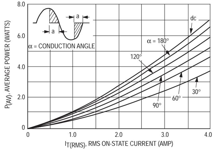
Figure 4. Power Dissipation
