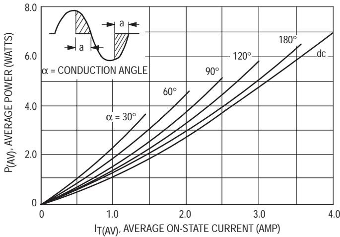
Figure 3. Power Dissipation
