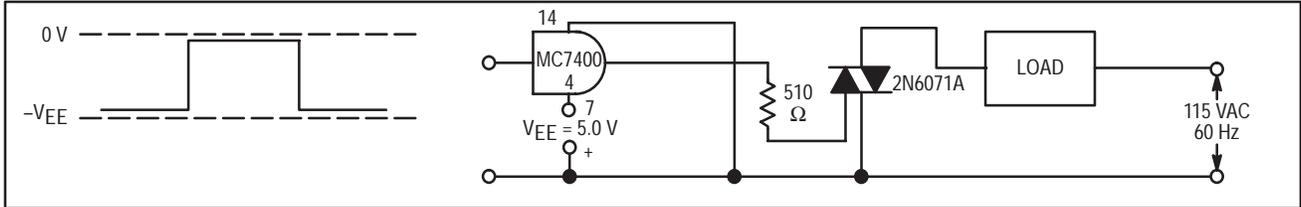
Trigger devices are recommended for gating on Triacs. They provide:
