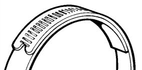
By pressing precisely formed serrations into the bands of strictly controlled 40—48 tons per sq. in. tensile steel a constant thread form is achieved which is further strengthened by work hardening.
