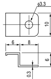
\*Mounting brackets exclusively for the OHD1 type are provided optionally (at separate cost).
