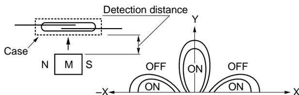
When drive magnet M approaches, the reed switch contacts close and the circuit comes on.
