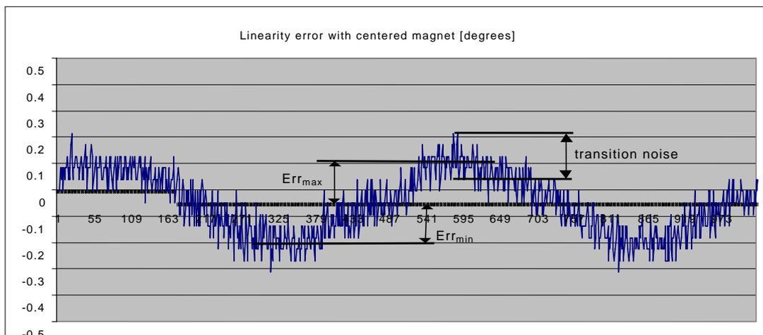
Figure 21: Example of linearity error over 360°
