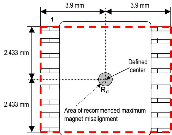
Figure 17: Defined chip center and magnet displacement radius
