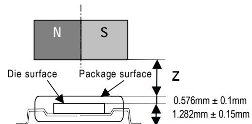
Figure 18: Vertical placement of the magnet
