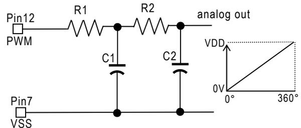
Figure 8: Simple 2<sup>nd</sup> order passive RC lowpass filter
