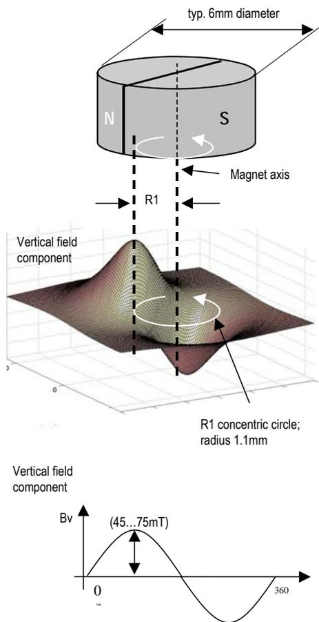
Figure 16: Typical magnet (6x3mm) and magnetic field distribution
