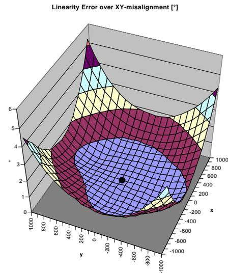
Figure 20: Example of linearity error over XY misalignment
