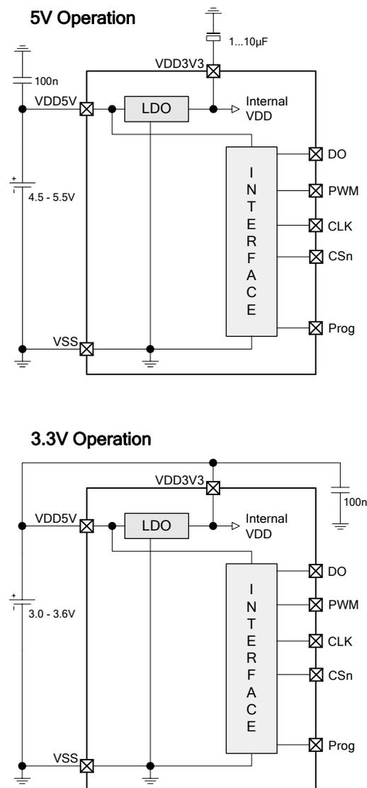
Figure 15: Connections for 5V / 3.3V supply voltages
