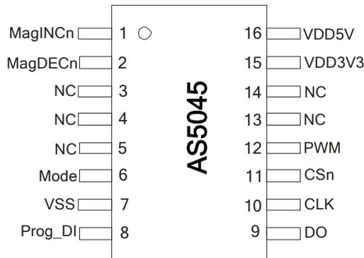
Figure 2: Pin configuration SSOP16
