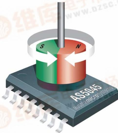
Figure 1: Typical arrangement of AS5045 and magnet
