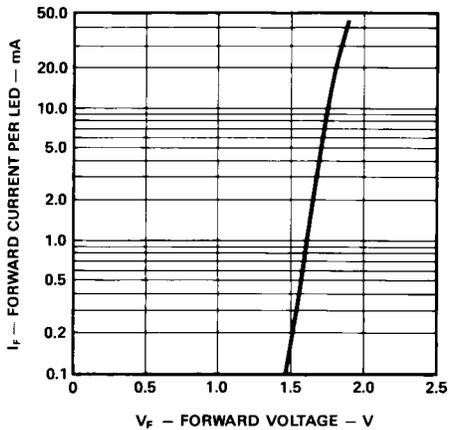
Figure 4. Forward Current per LED vs. Forward Voltage.
