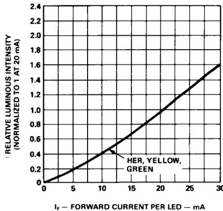
Figure 10. Relative Luminous Intensity vs. DC Forward Current.
