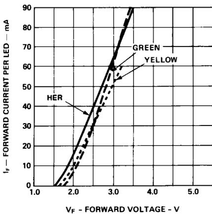
Figure 9. Forward Current vs. Forward Voltage Characteristics.
