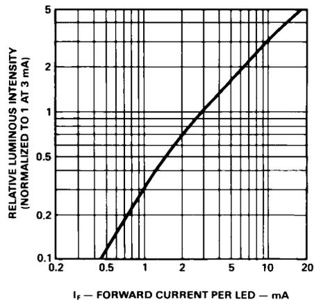
Figure 5. Relative Luminous Intensity vs. DC Forward Current.
