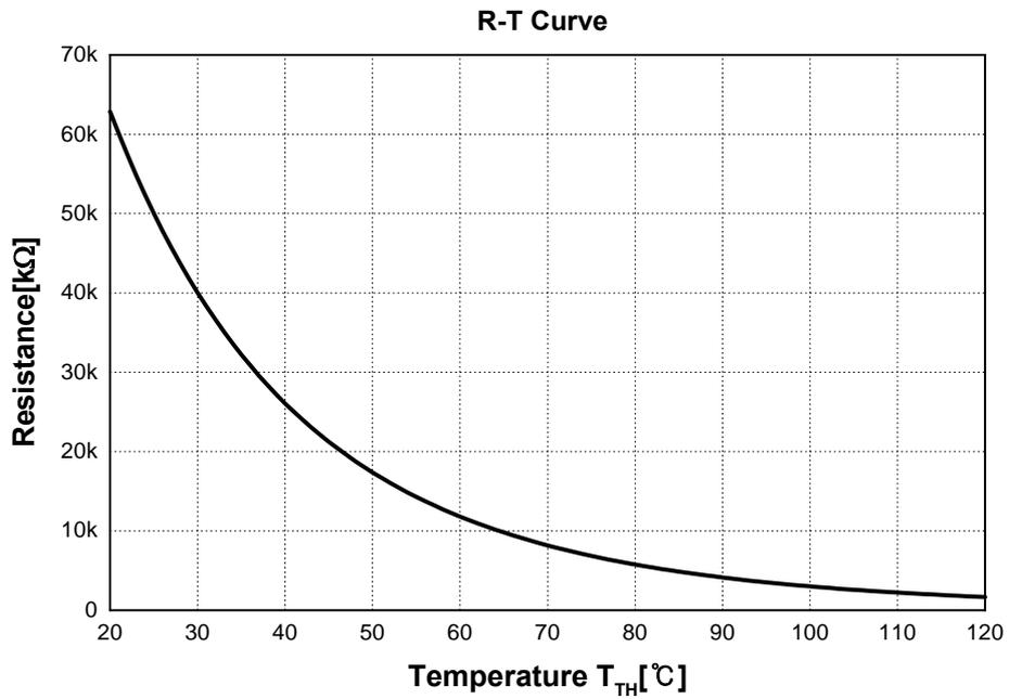
Fig. 5. R-T Curve of The Built-in Thermistor
