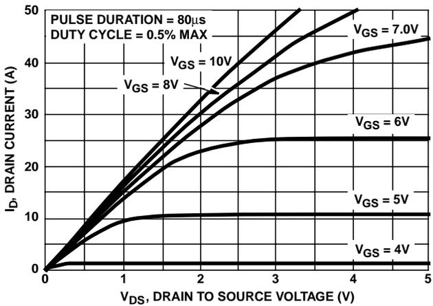
FIGURE 6. SATURATION CHARACTERISTICS
