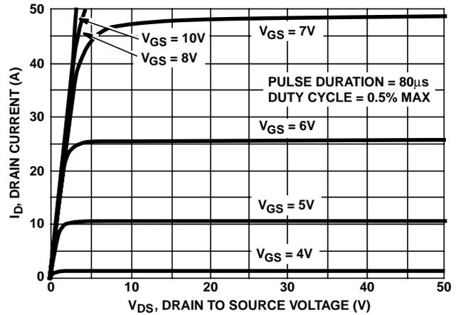
FIGURE 5. OUTPUT CHARACTERISTICS
