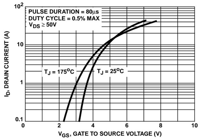
FIGURE 7. TRANSFER CHARACTERISTICS
