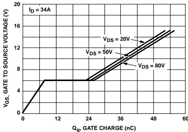
FIGURE 14. GATE TO SOURCE VOLTAGE vs GATE CHARGE
