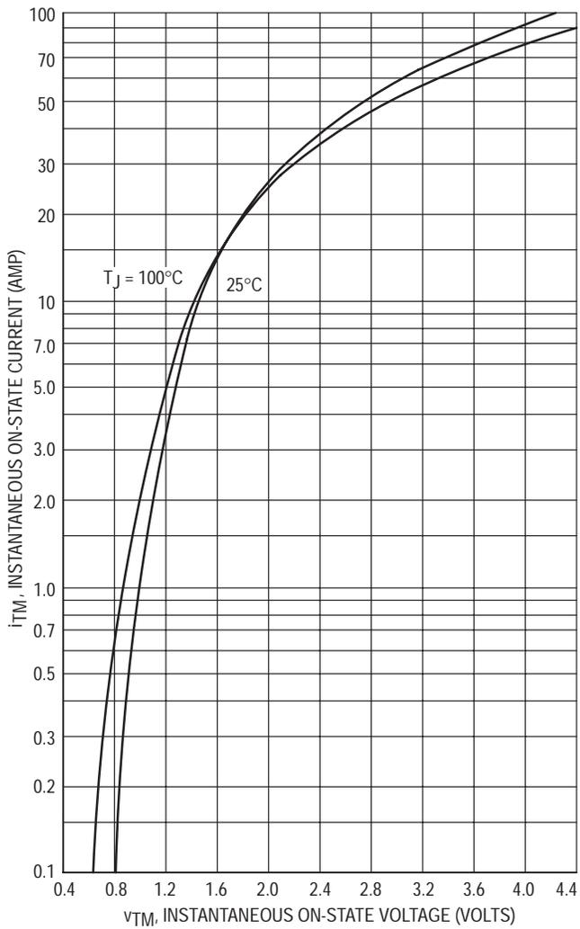
Figure 5. On-State Characteristics
