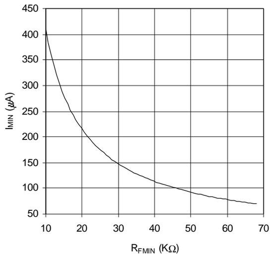
Graph 7. I<sub>MIN</sub> vs R<sub>FMIN</sub> (IR2159/IR21591)
