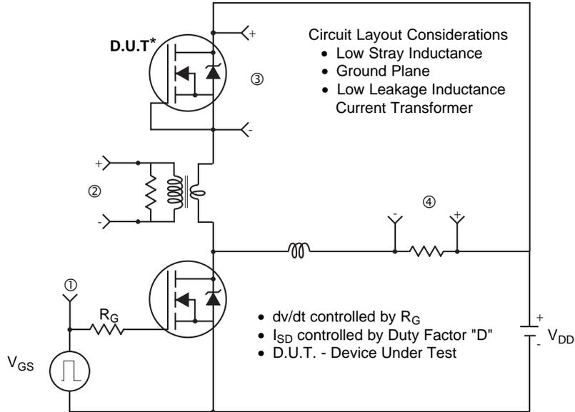
\* Reverse Polarity of D.U.T for P-Channel
