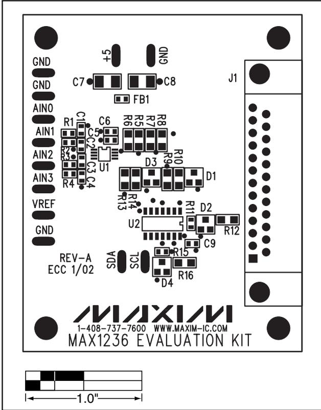
Figure 3. MAX1236 EV Kit Component Placement Guide—Component Side
