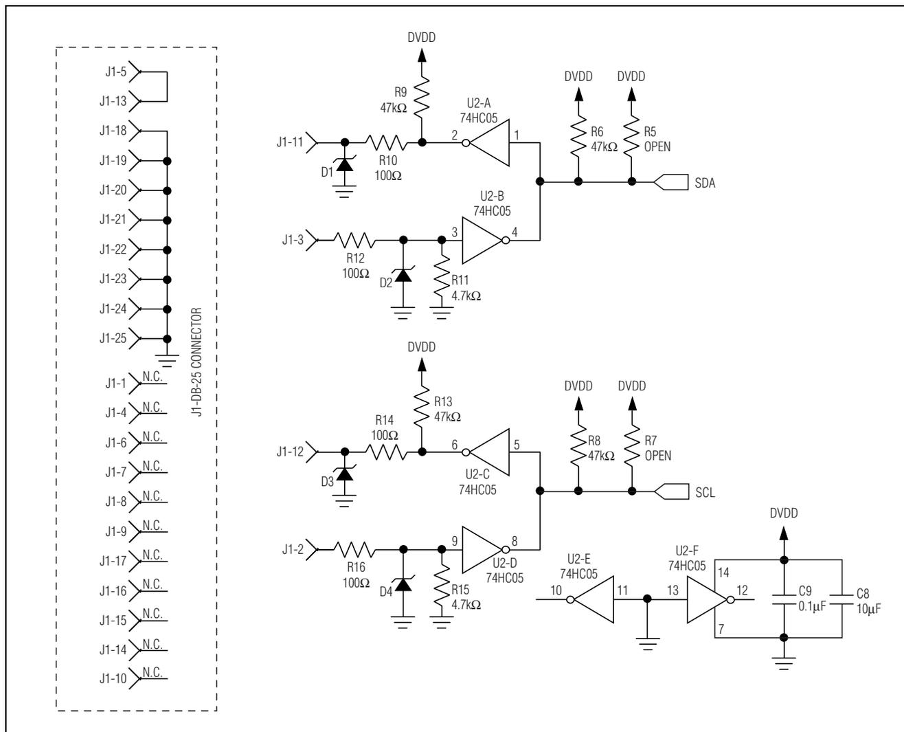
Figure 2. MAX1236 EV Kit Schematic (Sheet 2 of 2)
