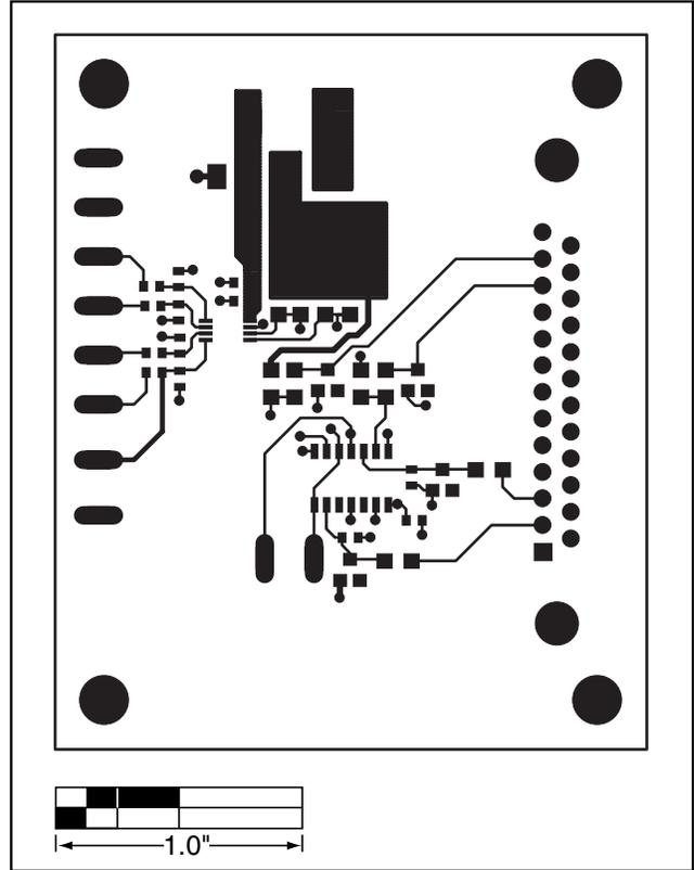
Figure 4. MAX1236 EV Kit PC Board Layout—Component Side
