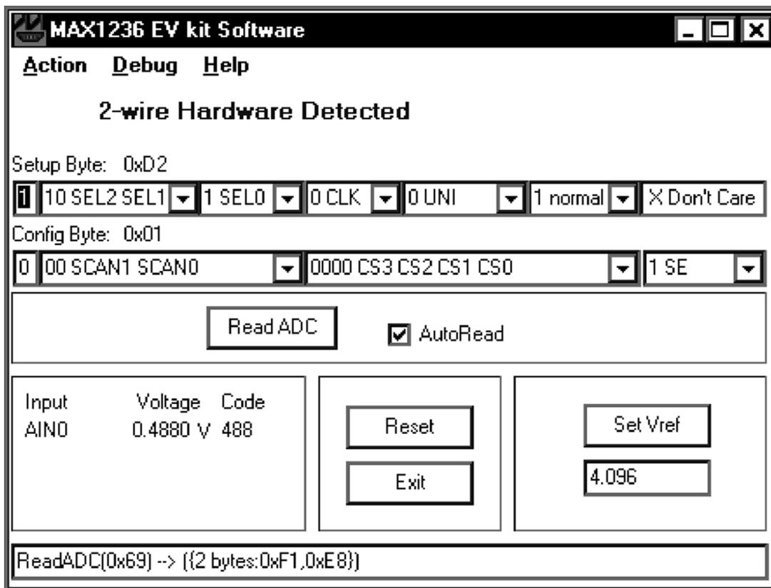
NOTE: MAX1236 EVALUATION SOFTWARE'S MAIN WINDOW CONTROLS THE MAX1236 AND DISPLAYS CONVERSION RESULTS.
