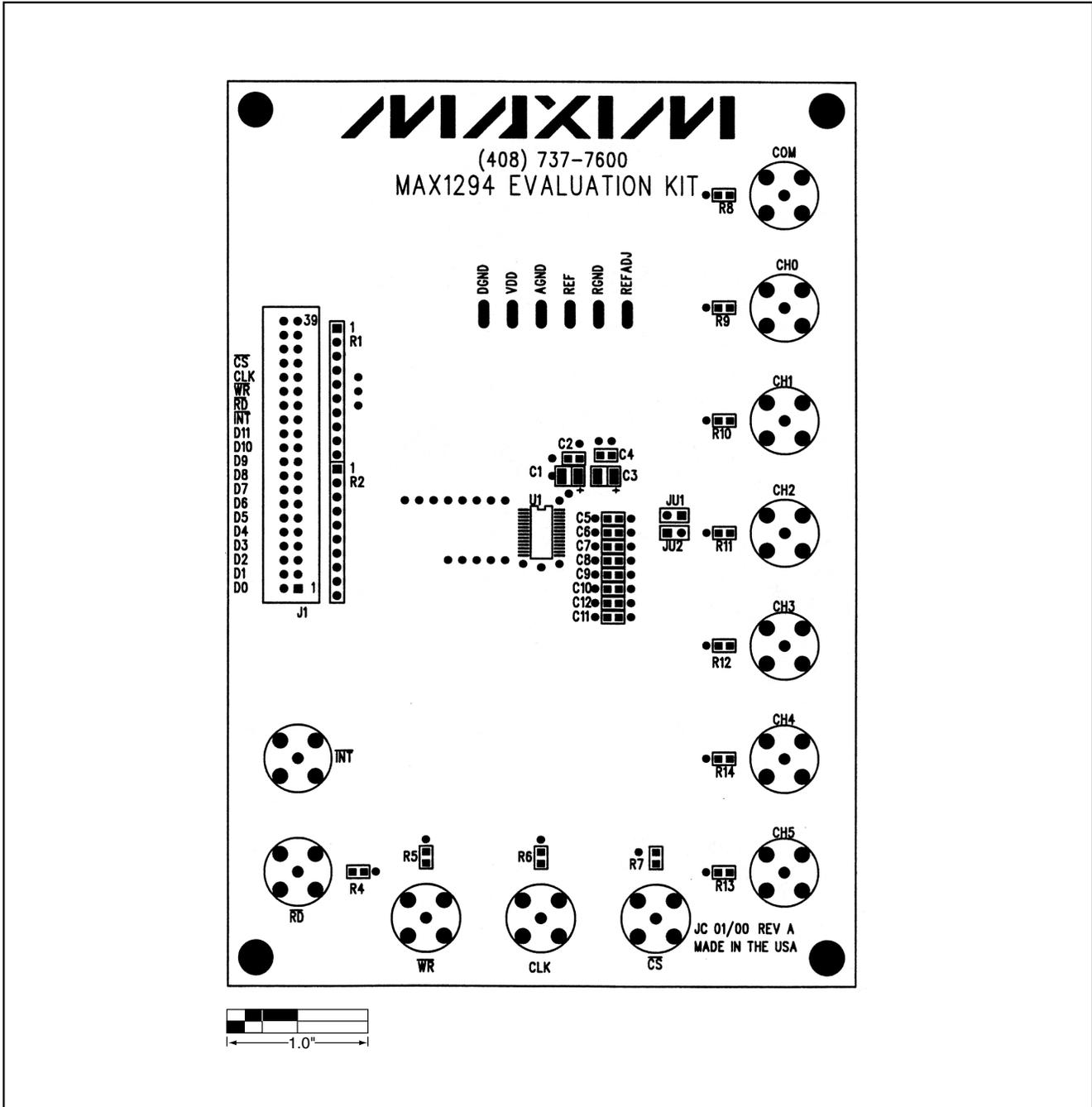
Figure 2. MAX1294 EV Kit Component Placement Guide—Component Side
