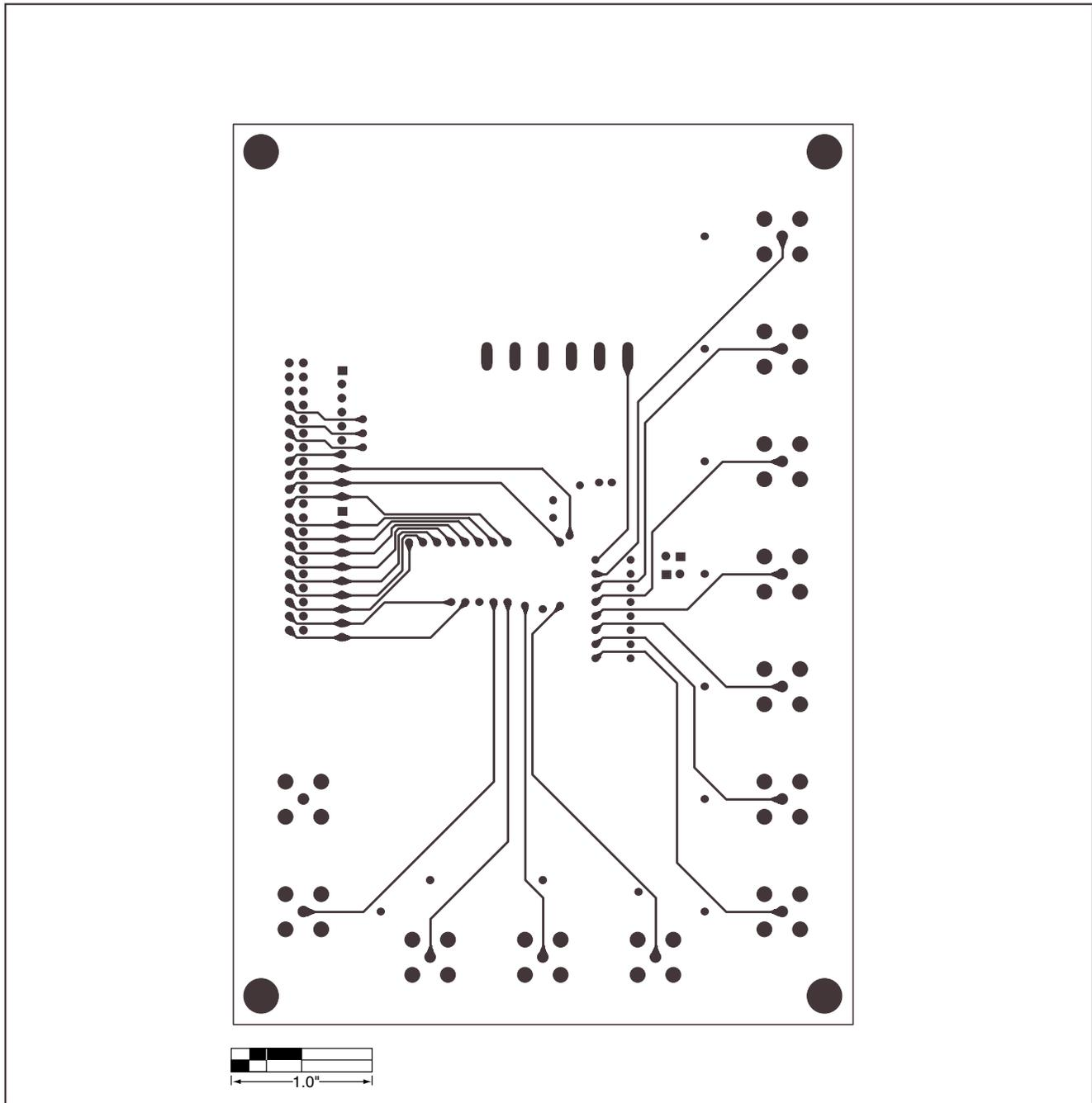
Figure 6. MAX1294 EV Kit PC Board Layout—Solder Side
