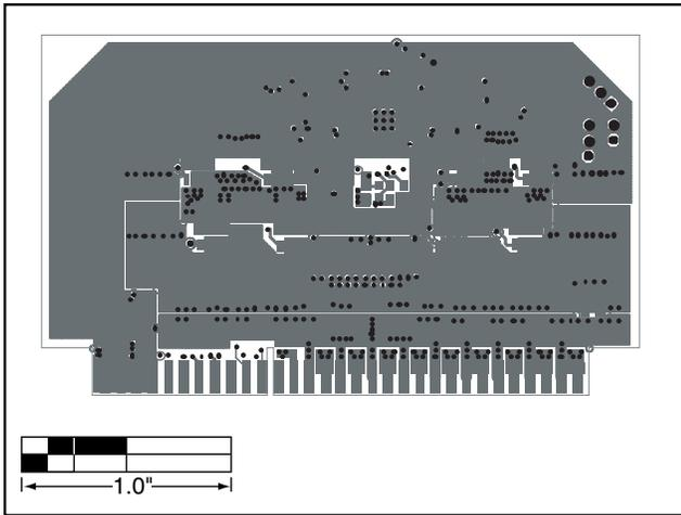
Figure 23. MAX5037 EV Kit PC Board Layout—Solder Side
