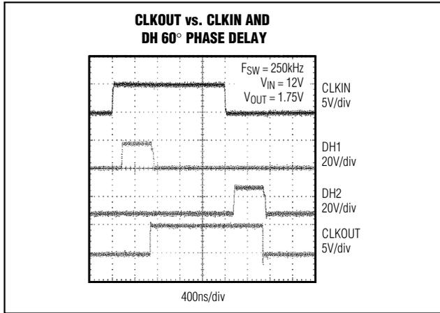
Figure 15. CLKOUT vs. CLKIN and DH 60° Phase Delay
