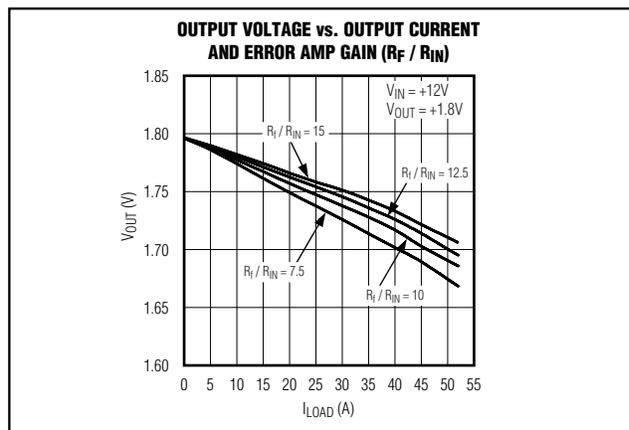
Figure 6. Output Voltage vs. Output Current and Error AMP GAIN (R<sub>F</sub>/R<sub>IN</sub>)
