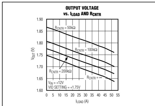
Figure 4. Output Voltage vs. I<sub>LOAD</sub> and R<sub>CNTR</sub>
