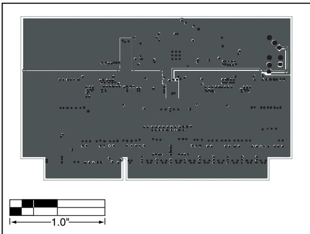
Figure 21. MAX5037 EV Kit PC Board Layout—Inner Layer 2
