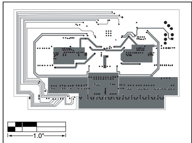
Figure 22. MAX5037 EV Kit PC Board Layout—Inner Layer 3
