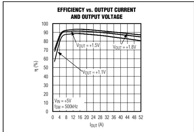
Figure 11. Efficiency vs. Output Current and Output Voltage
