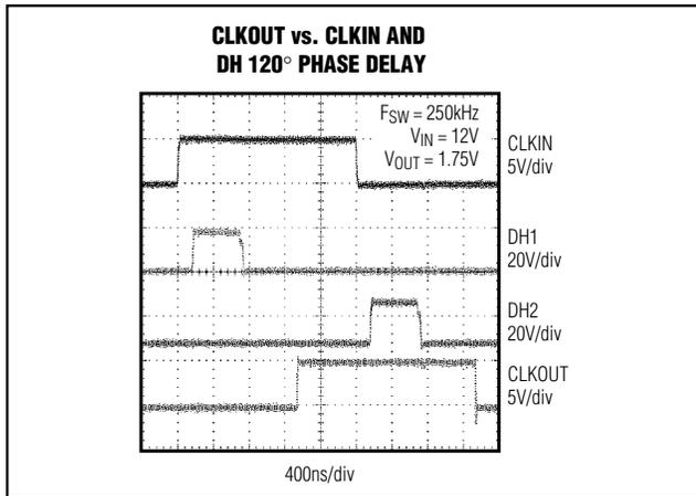
Figure 17. CLKOUT vs. CLKIN and DH 120° Phase Delay
