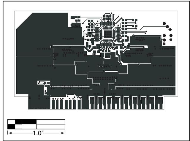
Figure 20. MAX5037 EV Kit PC Board Layout—Component Side
