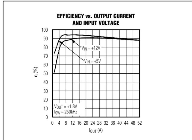
Figure 9. Efficiency vs. Output Current and Input Voltage
