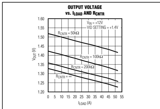
Figure 5. Output Voltage vs. I<sub>LOAD</sub> and R<sub>CNTR</sub>
