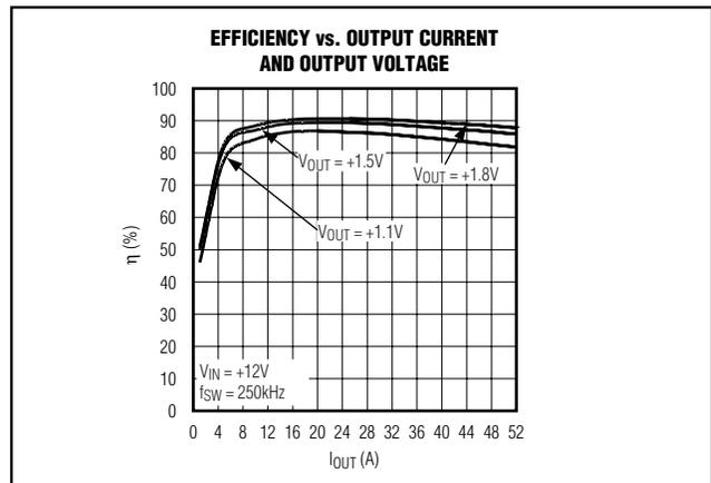
Figure 10. Efficiency vs. Output Current and Output Voltage
