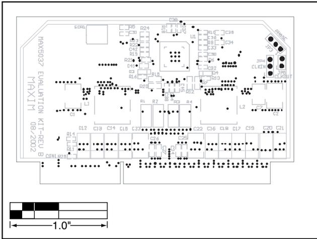
Figure 19. MAX5037 EV Kit Component Placement Guide—Component Side
