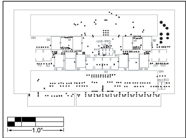
Figure 24. MAX5037 EV Kit Component Placement Guide—Solder Side
