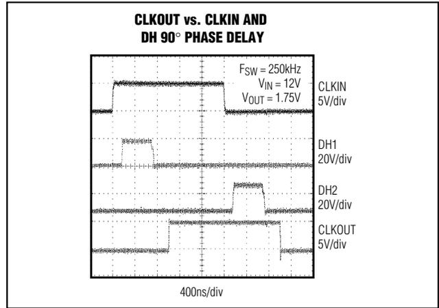
Figure 16. CLKOUT vs. CLKIN and DH 90° Phase Delay
