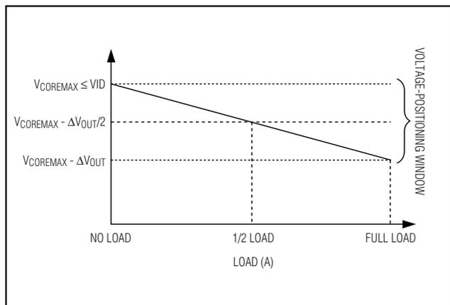
Figure 3. VRM Loadline with V<sub>COREMAX</sub> = VID at No Load
